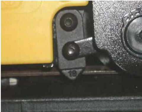
**2.** Pull the feedwheel handle (#58) toward the sealing handle (#73) with your right hand. While in this position, insert the strap into the sealing section against the front strap stop (#13) so the strap sits inside the side strap stop (#91 or #92). The end of strap should protrude 1" beyond the front strap stop (#13). Release the feedwheel handle (#58) so the strap is locked and ready to be tightened.
