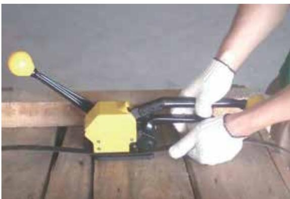
1. Feed the strapping around the package and hold in place with left hand. The end of strap is underneath.
