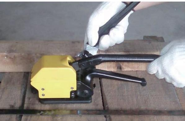
**5.** Move the sealing handle (#73) back to its original position. Hold the cut off strap end with the left hand. Lift the feed wheel handle (#58) toward the sealing handle (#73) to release the strap. Slide the tool away to the right.
