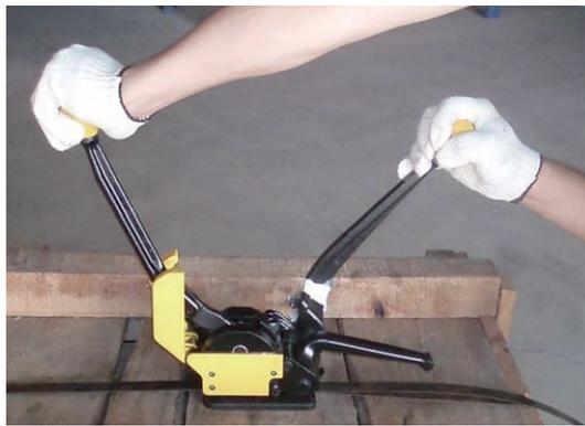
**4.** Place right hand firmly on the tensioning handle (#82) for supporting the tool. Move the sealing handle (#73) all the way forward until it hits the stop (#51). This seals and cuts the strap.
