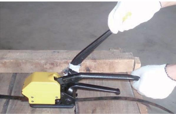
**3.** Hold the sealing handle (#73) firmly with left hand. Pump the tensioning handle (#82) with your right hand until the desired tension is reached.
